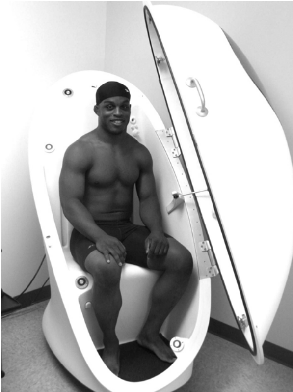
Figure 1. Body composition analysis using the Bod Pod® Body Composition System (Life Measurement Instruments, Concord, CA)
