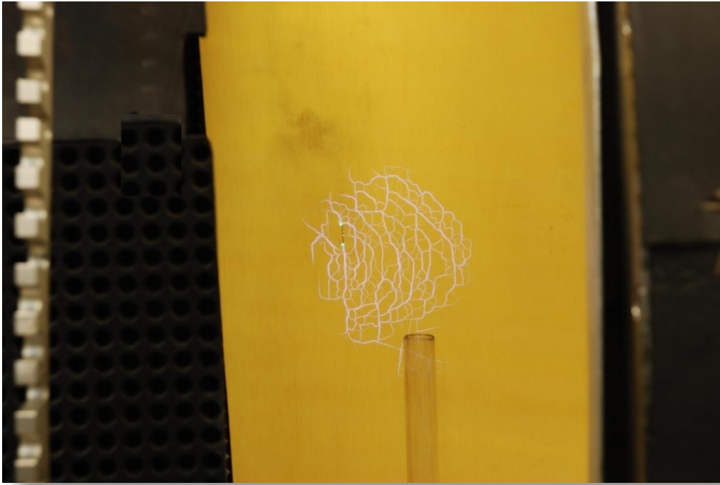
Fig.9.1. Experiment formulation: initiated surface MW discharge on the textolite plate and the quartz tube for propane-air mixture injection
