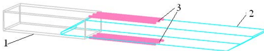
Fig.11.22. Systems with a discharge model: 1 – a waveguide, 2 - antenna, 3 – thin rods simulating the streamer discharge.
