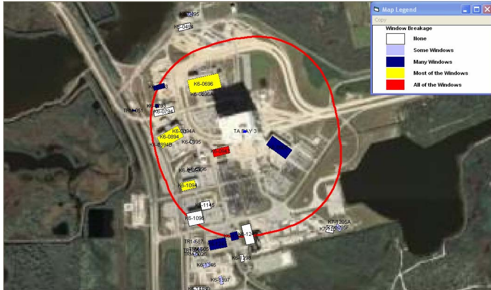
Figure 15. Window Breakage due to Air Blast.
