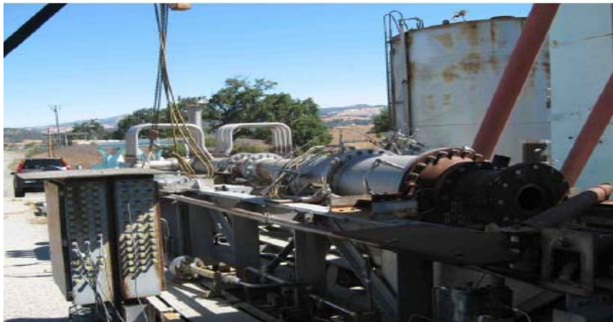
Figure 2. RT-6 Vitiator and Air Lines
