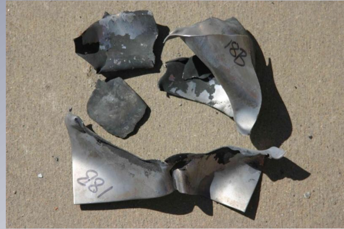
#8 Vertical Tear (Positive) – 1 Trial (Fail)
