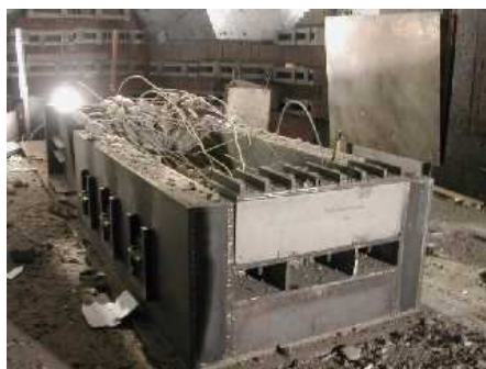
(a) Clamped slab test
