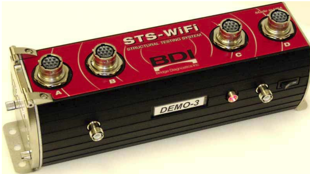
Figure D2. BDI structural testing system.
