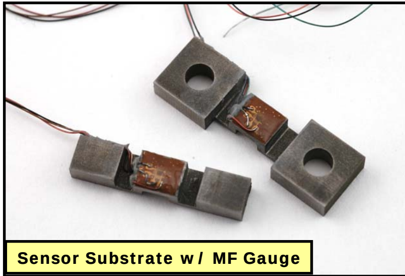
Figure DS2: GEN-2 displacement sensor w/ metal-foil strain gauge
