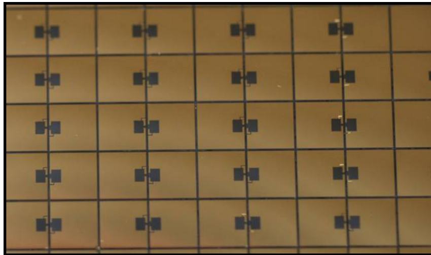
Figure SS7: Backside wafer-level Au / Sn patterning
