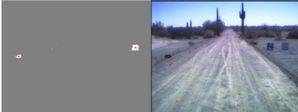
Figure 2. Target declaration from binary mask. Red dots are target declarations.
