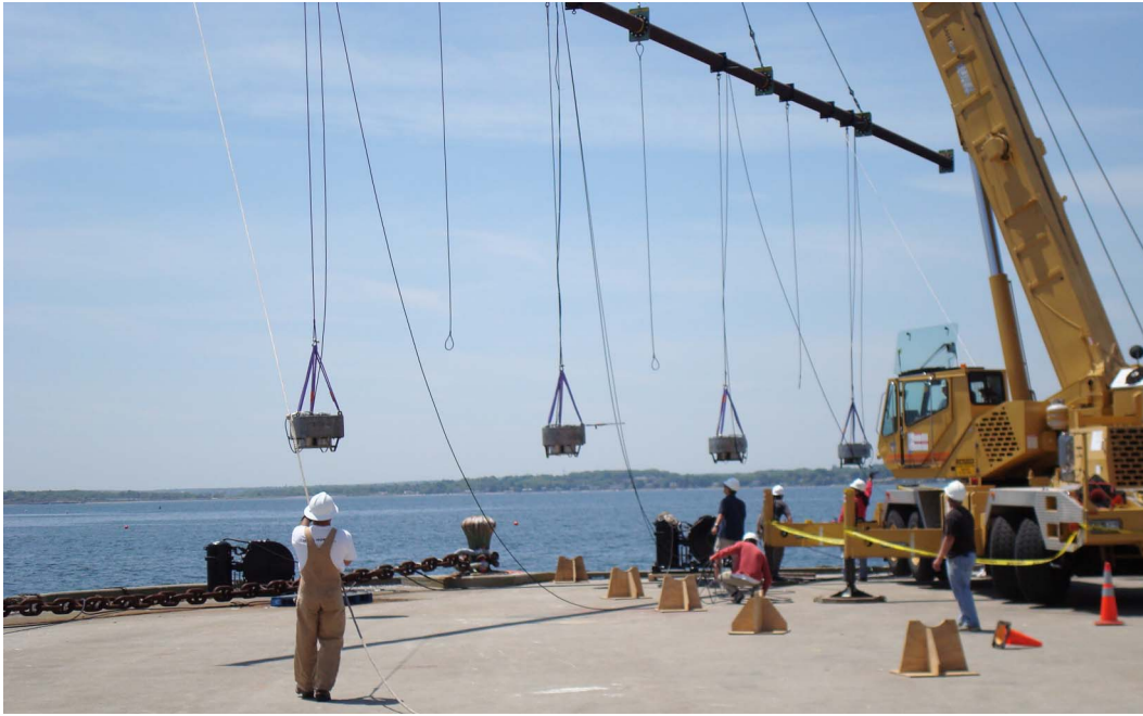
Fig. 1 Source fixture suspended above pier with 4 J-15-3 low-frequency projectors.
