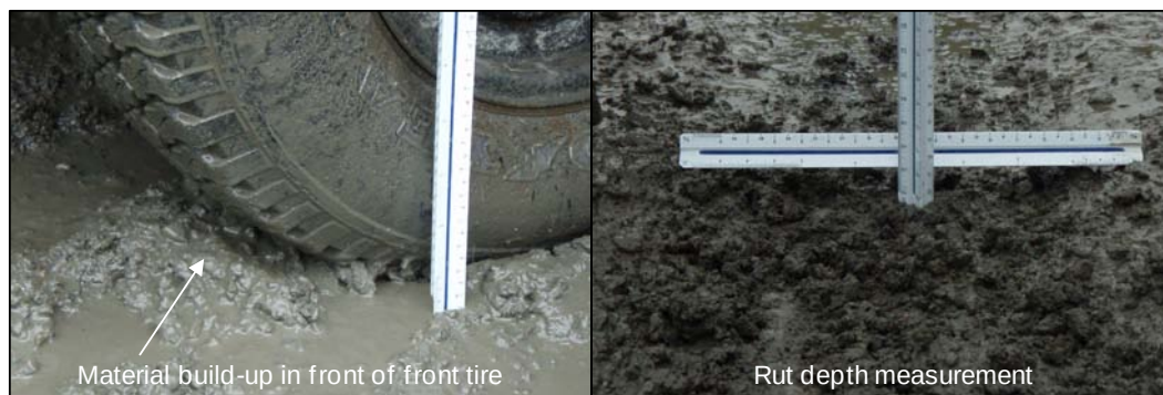
Figure 5. Material buildup in front of front tires and rut depth measurements.
