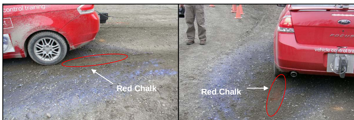
Figure 3. Second SLB test with Ford Focus at Team O'Neil — Red Chalk from the deeper layers is visible behind rear tire after a second SLB test in the same vehicle path.
