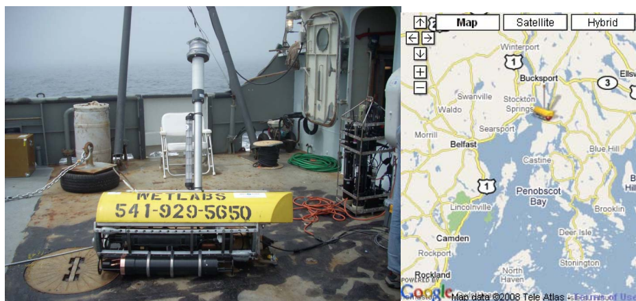
Figure 2. Left panel: Picture of the Penobscot Bay LOBO monitoring system on deck of the RV Argo ready to deploy. Sampling instrumentation, WET Labs WQM, FLCDS, Satlantic ISUS, and Sequoia LSST are mounted on the frame below the yellow flotation. Right panel: Map of the upper Penobscot Bay with the deployment location of the LOBO mooring shown as a yellow icon. The mooring is located south of the town of Bucksport, ME. Map courtesy of Google Earth.
