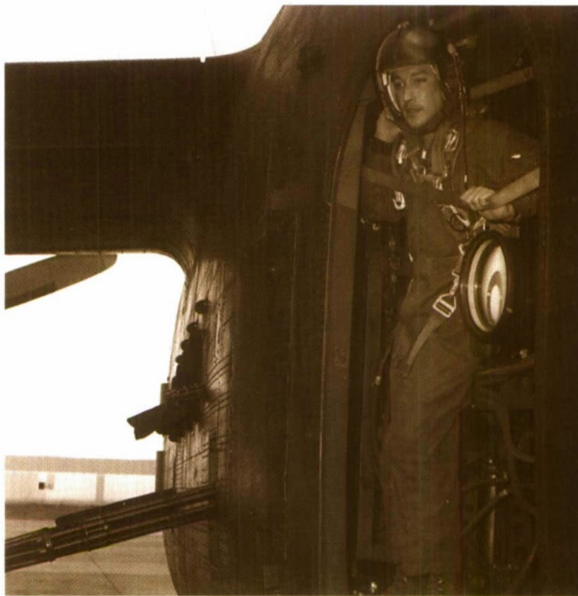
USAF The 1.5-million-candlepower variable-beam illuminator shown here could light up a football field-sized area with brilliant white light. Of course, it also made the gunship a beautiful target for anti-aircraft gunners determined to rid themselves of such unwanted visibility.
