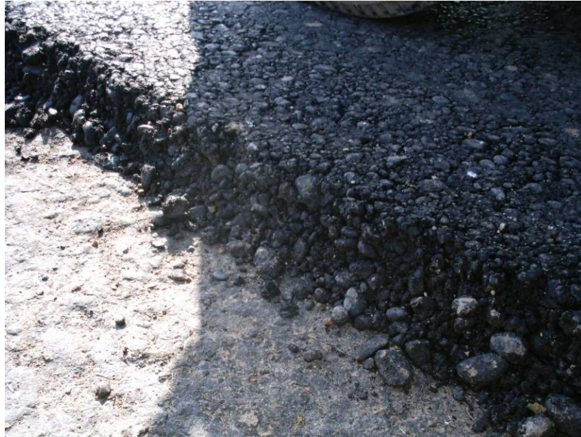
Site Photo 8. Uncrushed gravel used in the asphalt mix (USACE photo taken 18 Dec 05)
