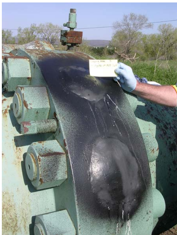
Figure 5-68. Press 15, one week after BTS application, prior to sampling.
