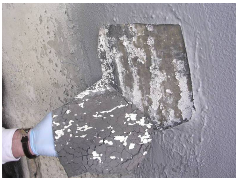
Figure 5-41. One week post application, during sampling, Mg/Pd-silicon, 6810-11.
