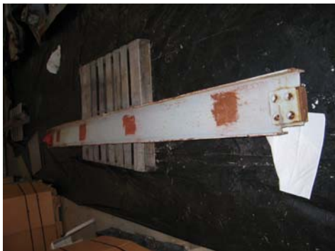
Figure 5-7. Test I-Beam 8 prior to application of BTS
