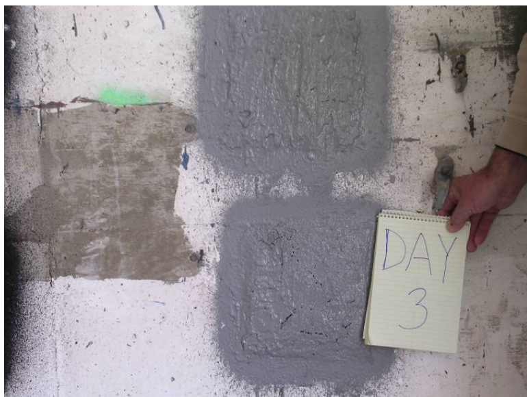
Figure 5-21. Mg/Pd-Sil, three days after treatment, 6810-36.
