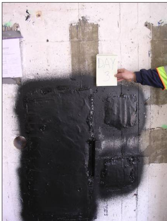
Figure 5-20. Mg/Pd-VP test location after three days of treatment, 6810-36.
