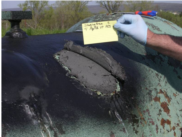
Figure 5-66. Treatment areas on press 4 one week after BTS application, prior to sampling.
