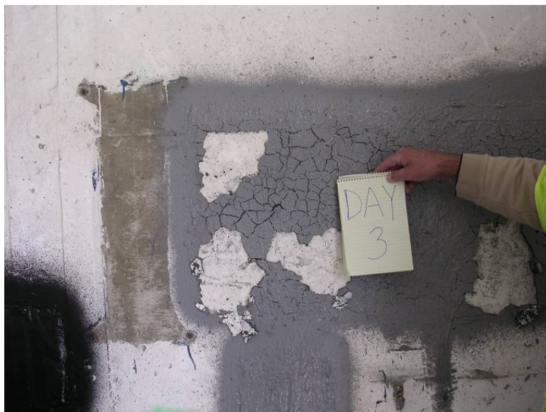
Figure 5-22. Mg/Pd-Sil, three-foot section, after three days of treatment, 6810-36.
