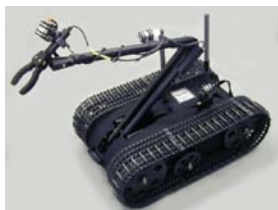
(a) Talon - Used for reconnaissance to weapons delivery (Global Security 2000)
