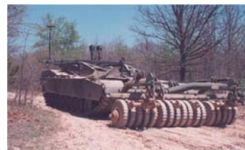
(c) Panther II - Remote controlled tank used for mine clearing missions (Global Security 2000)
