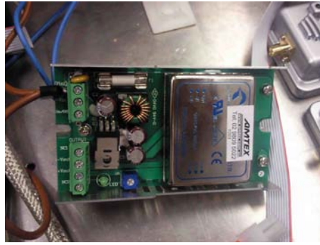
Figure 3.32: An example of one DC/DC converter
