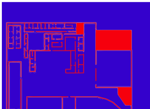
Figure 8.9: The elevation map displayed on the HMI. The elevation of ground level in the occupancy grid is displayed as blue and elevations above ground are displayed as shades of red where a brighter red indicates a higher elevation.
