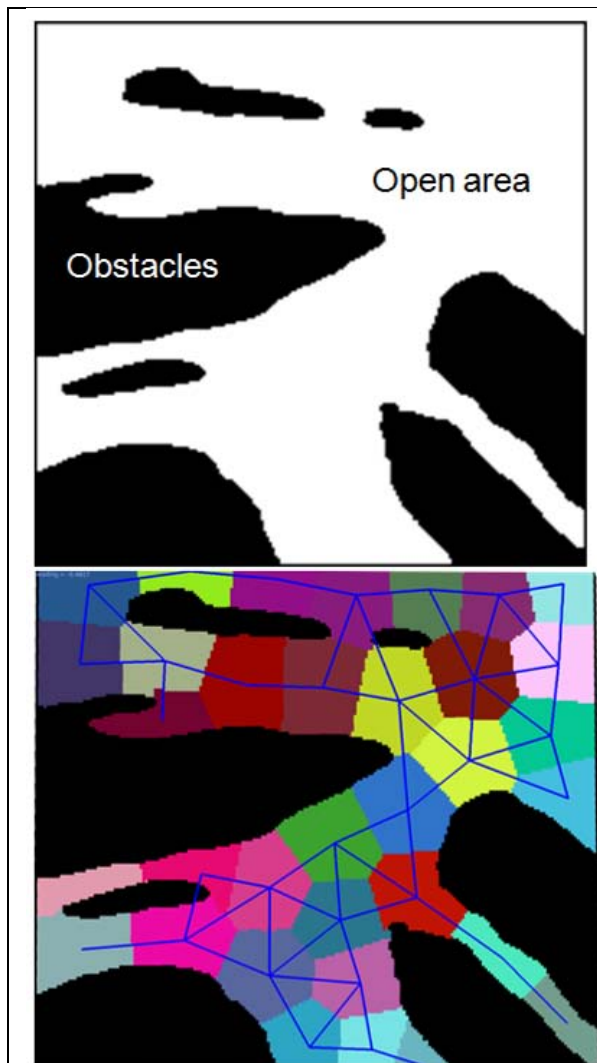
Figure 6. KML automatically subdivides the total area into smaller areas called “countries”, each with a “capital”. From the capital the robot can see the entire country, given the known obstacles.
