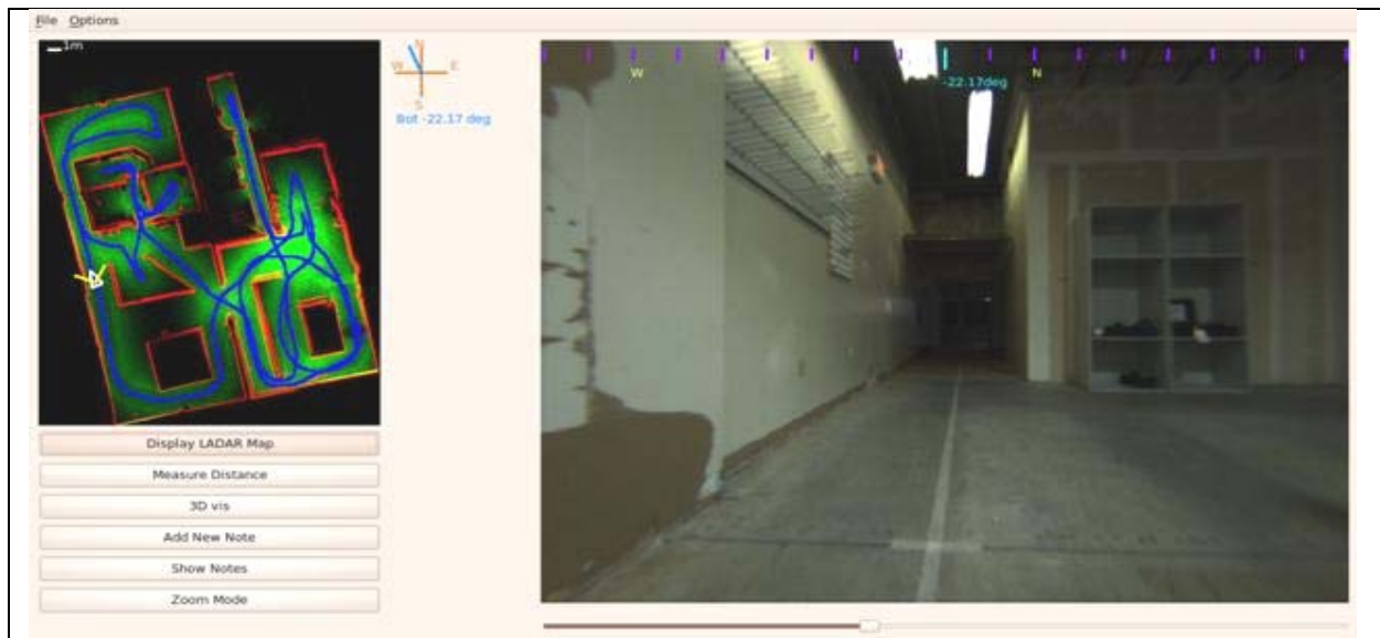
Figure 12. RR-Viewer allows the operator to pan, tilt, zoom and teleport to navigate the scene. 2D and 3D maps are available as well image recall and playback from prior locations similar to Google's Streetview system.
