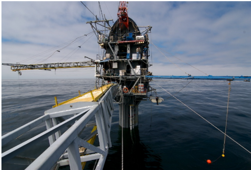
Figure 1: R/P FLIP deployed on the south of Monterey Bay during AESOP. The port boom, on the left, supported the Deep 8 Doppler system; the aft boom, in the foreground, supported the fastCTD. (Photos: T. Hughen)
