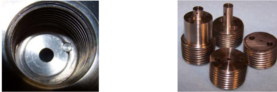
Figure 3: (Left) Threading for installation of interchangeable flash-tube vent section (installed flash tube section with steel alignment pin also shown). (Right) Interchangeable flash-tube vent sections with various orifice configurations.
