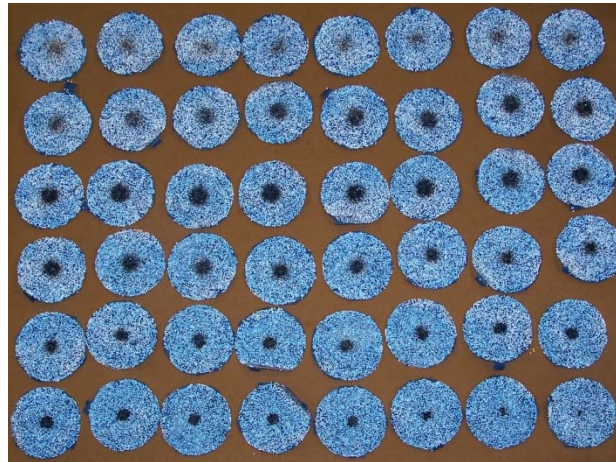
Figure 18: Series of removed inert layers, the top left is closest to the orifice.
