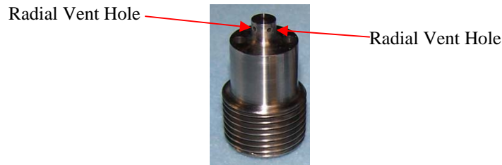
Figure 11: Flash-tube vent section with four axi-symmetric, radial vent holes used for the axial flame-spreading experiments.
