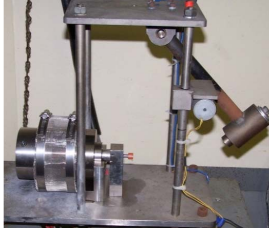
Figure 10: Radial/Azimuthal test rig configuration installed on test stand at HPCL.
