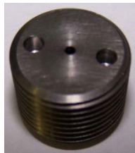
Figure 13: An interchangeable flash-tube vent section with an axial jet configuration used in the condensed-phase deposition experiments.
