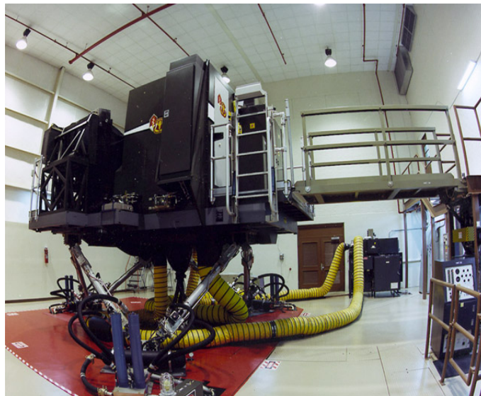
Figure 2. The USAARL NUH-60 research flight simulator.
