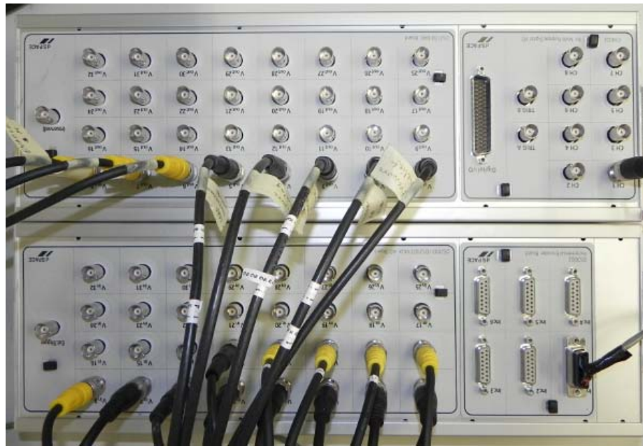
Figure 4.6. Picture of I/O box for the experimental setup. Top box has a D/A converter and a digital I/O, while the bottom box hosts A/D converters.
