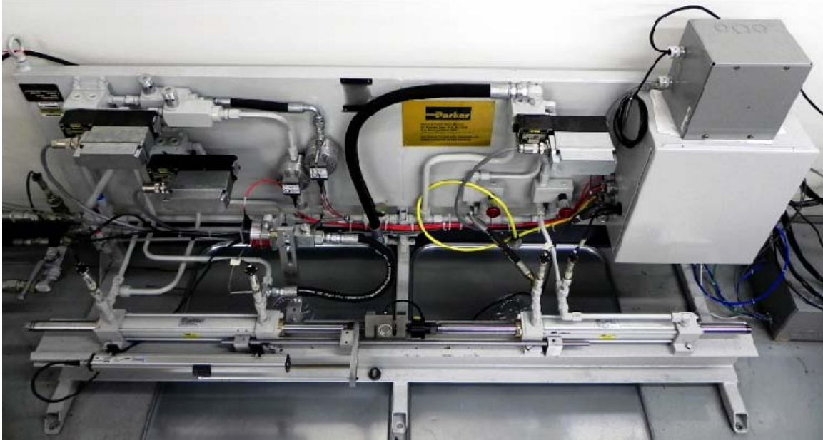
Figure 4.5. Picture of the experimental test bench showing both the load (right of the center) and actuator circuits (left of the center). The load and actuator cylinders are connected with a load cell.
