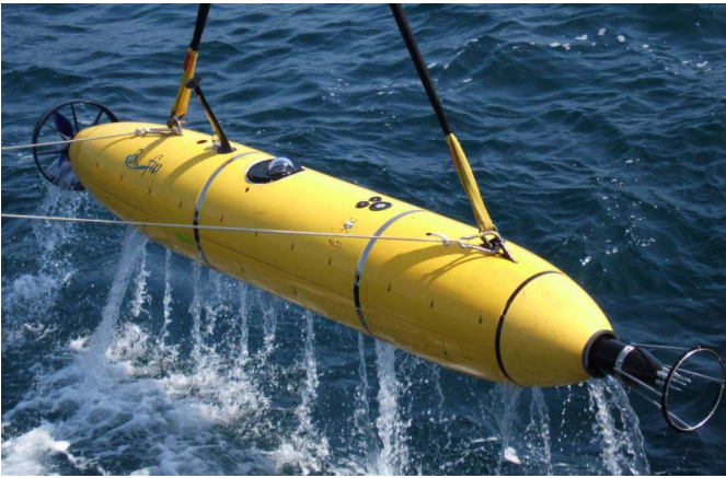
Figure 1: Photographs of three RadCam instruments are a) the in-air reference camera mounted on a tripod on the roof of the lab on the pier at Scripps, b) the logging camera mounted on a cage and being lowered into the water c) the logging camera mounted on an AUV (center of Bluefin) and d) the profiler camera system hanging from the wire as it is being deployed in the ocean off Santa Barbara, CA.
