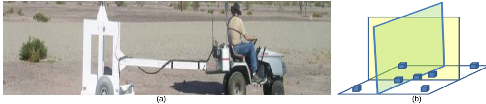
Fig. 2. (a) MetalMapper system being towed by a tractor, (b) Schematic of a MetalMapper sensor array, where three mutually orthogonal squares represent three transmitters and blue cubes in the horizontal plane represent the multi-axis receiver arrays.
