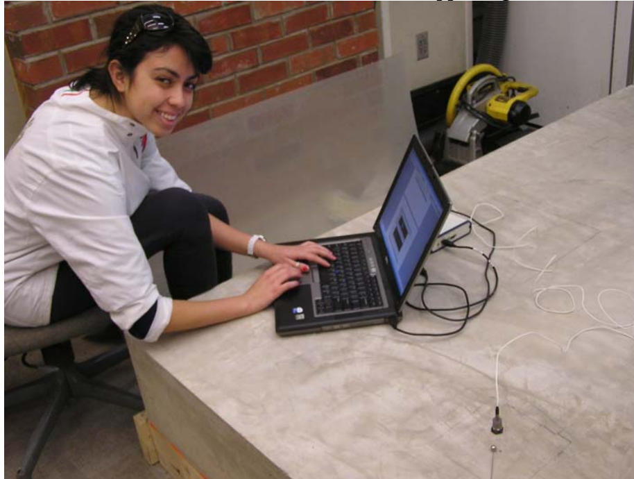
Figure 1: Accelerometer testing of a test slab, including operator, computer, data acquisition module (partially concealed behind computer and accelerometer).
