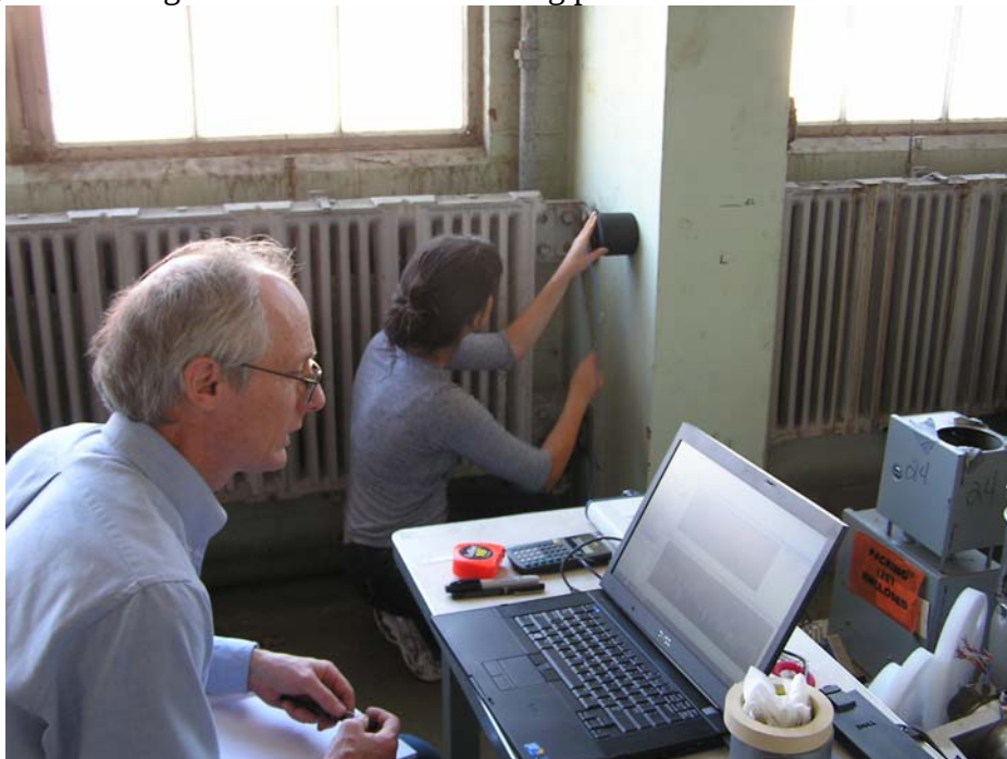
Figure 12: Air-coupled impact-echo testing of pedestal in Building 19.
