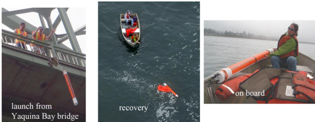
Figure 1 – Impact tests. Inertial motion package dropped from Yaquina Bay bridge. This was repeated many times with different parachutes and internal sensor configurations.
