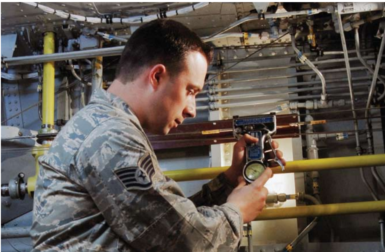
SSgt Greg Thompson uses a cable tension meter to check an aileron cable inside the main landing gear wheel well on a KC-135 Stratotanker at March Air Reserve Base, California.
