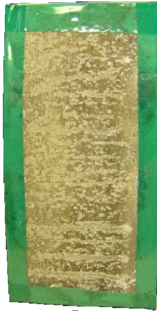
Figure 9. Optical images of coated aluminum 7075-T6 panels after exposure to salt fog for 18 hours A) chemical immersion, B) chemical wipe, C) ultrasonic processing, and D) abrasive blasting.
