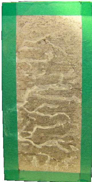
Figure 8. Optical images of prepared, uncoated aluminum 7075-T6 panels after exposure to salt fog for 18 hours A) chemical immersion, B) chemical wipe, C) ultrasonic processing, and D) abrasive blasting.
