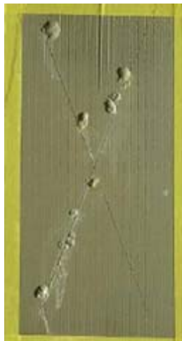
Figure 41. Optical image of a Round 2 Hybricor 204 MUV coated Al 2024-T3 panel that did not have a conversion coating (bare) after 2000 hours salt spray.
