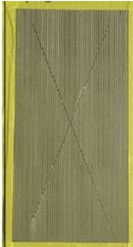
Figure 40. Optical image of a Round 2 Hybricor 204 MUV coated Al 2024-T3 panel with a TCP conversion coating after 2000 hours salt spray.
