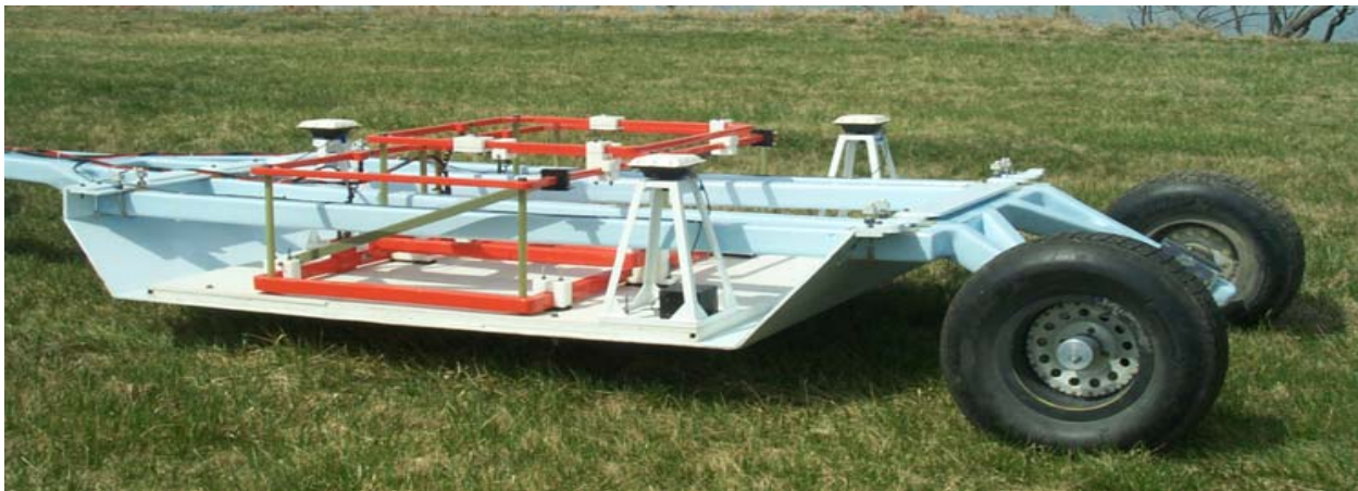
Figure 8. Close-up of EM61MTADS array with GPS and IMU.
