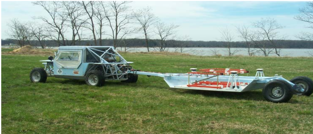
Figure 6. EM61MTADS array pulled by the MTADS tow vehicle.
