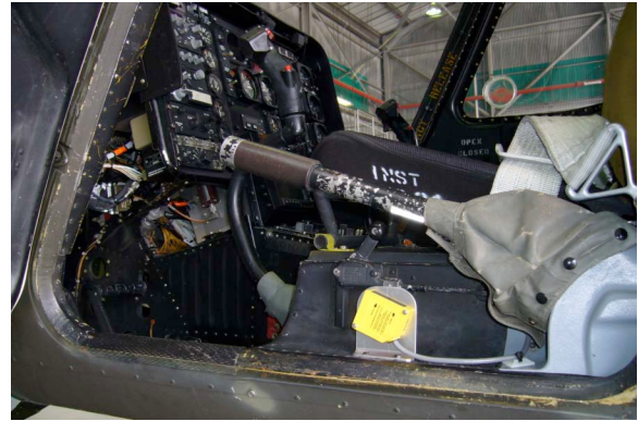
Figure 3. Collective lever with non-intrusive reflector on stick and floor-mounted infrared position sensor.
