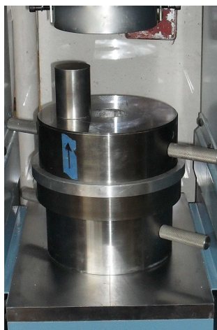
Figure 3.1: Pore solution extraction device inside compression testing machine
