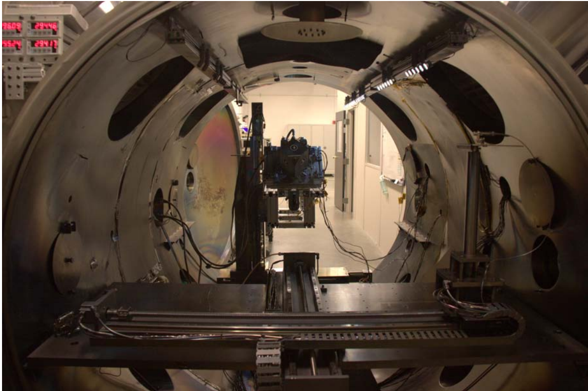
Figure 17: Beam profiler translation stage is in the foreground. The three-axis thruster is mounted to the Aerotech translation stage at the far end of the chamber.
