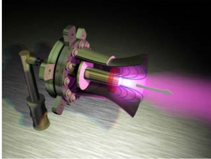
Figure 3: Schematic of a magnetoplasmadynamic thruster, from NASA Glenn Research Center [7].
