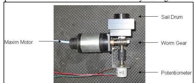
Fig. 10 In-house worm gear winch.
