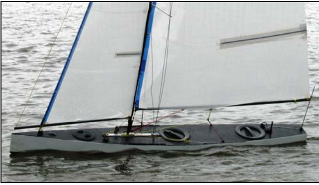
Fig. 3 Boat 2 showing mast step and rigging details.
