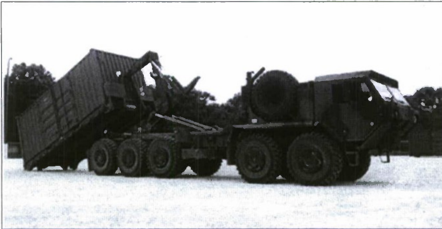
Figure 4.2 HEMTT PLS Loading a Standard Container
