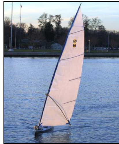
Fig.1 Freestanding Rig 4 with wishboom on Boat #2
