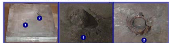
(a) Damage of the ceramic face plates
