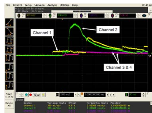
Figure 15 Response signals from the blast tube test
