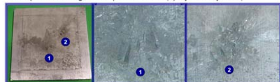
(b) The top surface damage of back plates
