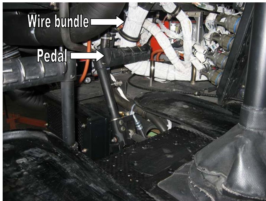
Figure 1 Left seat pedals versus wire bundles routing
