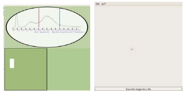
Fig. 5. The selected BGO crystal and the energy spectrum of the BGO detector, left. The estimated position of the single NaI pixel, right.
