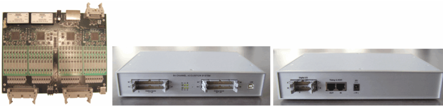
Figure 9. Fast FPGA-based multi-channel DAQ electronics circuitry developed by James Proffitt (now at AiT). One 64 channel system like this would read all the channels of the dedicated prostate PET system (panel+probe).
