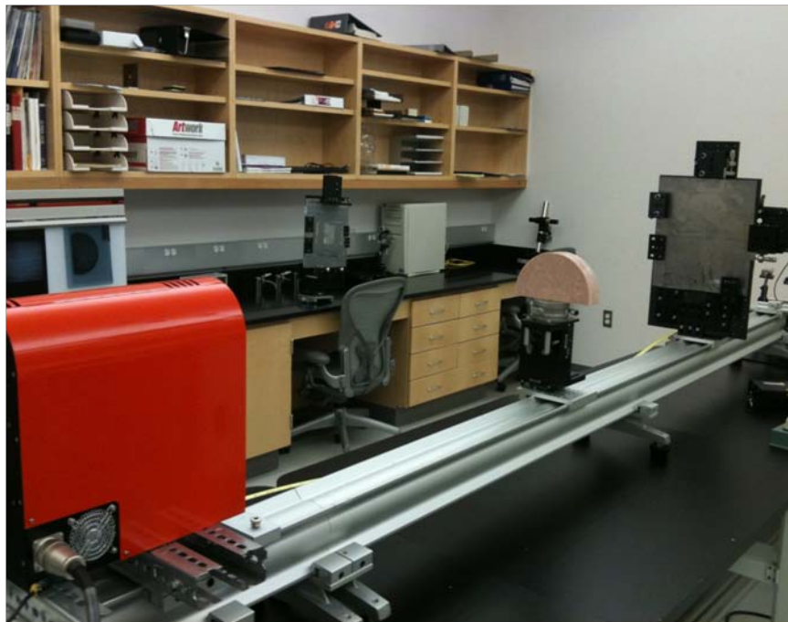
Fig. 5. A high energy x-ray phase contrast imaging system
