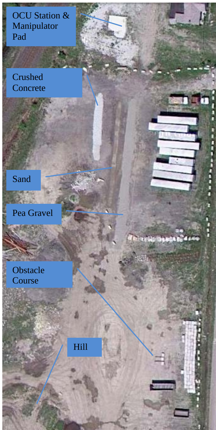
Figure 4 – Overhead View of Test Site
