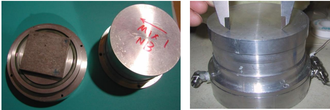
Figure 3. Photos of the Al sample holder used in D 2 O-vapor-conditioning experiment.
