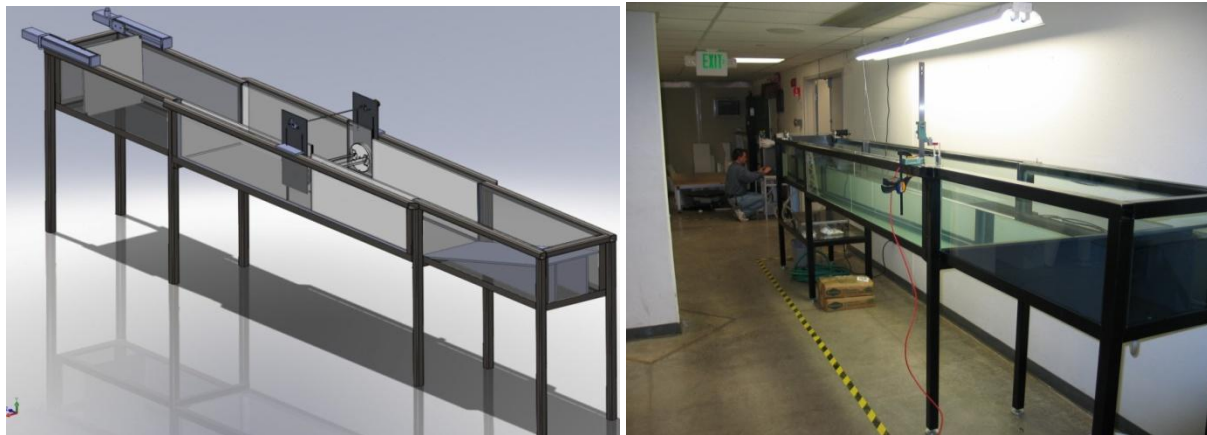
Figure 32: Conceptual design of the wave tunnel and operational wave tunnel.
