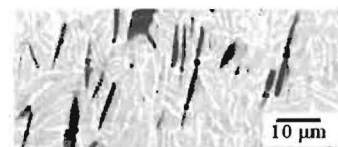
Figure 7. BSE image of the interior TiB cracking evident in the RT deformed sample in Figure 5 after failure just behind the fracture surface.
