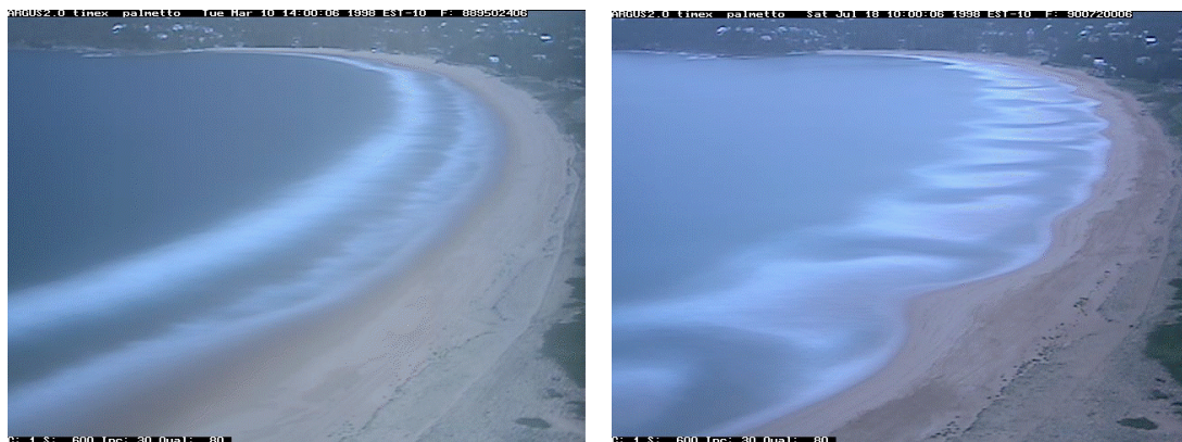
Figure 1 Time exposure images from the new colour camera installed in January 1998. The left panel shows the Longshore Bar-Trough morphology while the right panel shows Transverse Bar and Rip morphology as defined by Wright and Short (1984).
