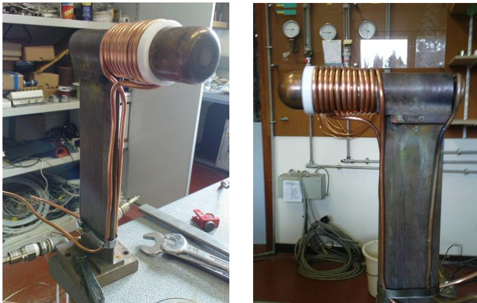
Figure 3-3: The standard (left) and hemispherical (right) heat flux probes
