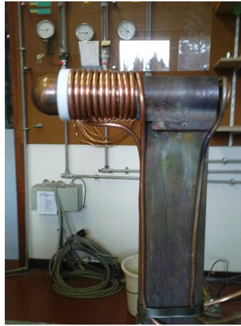
Figure 3-6: The hemispherical heat flux probe with the cooling spiral and ablative ring
