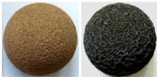
Figure 5-3: Amorim P50 samples before (left) and after (right) test
