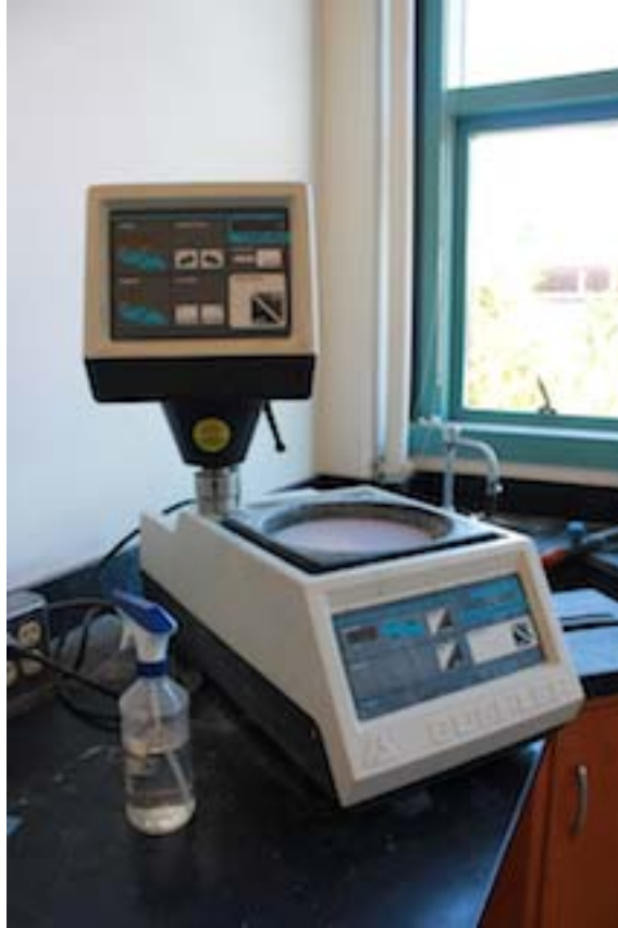
Figure 23. Buhler rotating wheel used for lapping of samples.
