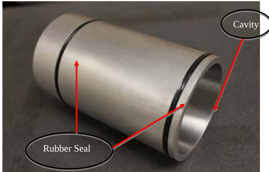
Figure 21. Aluminum alloy 6061 projectile
