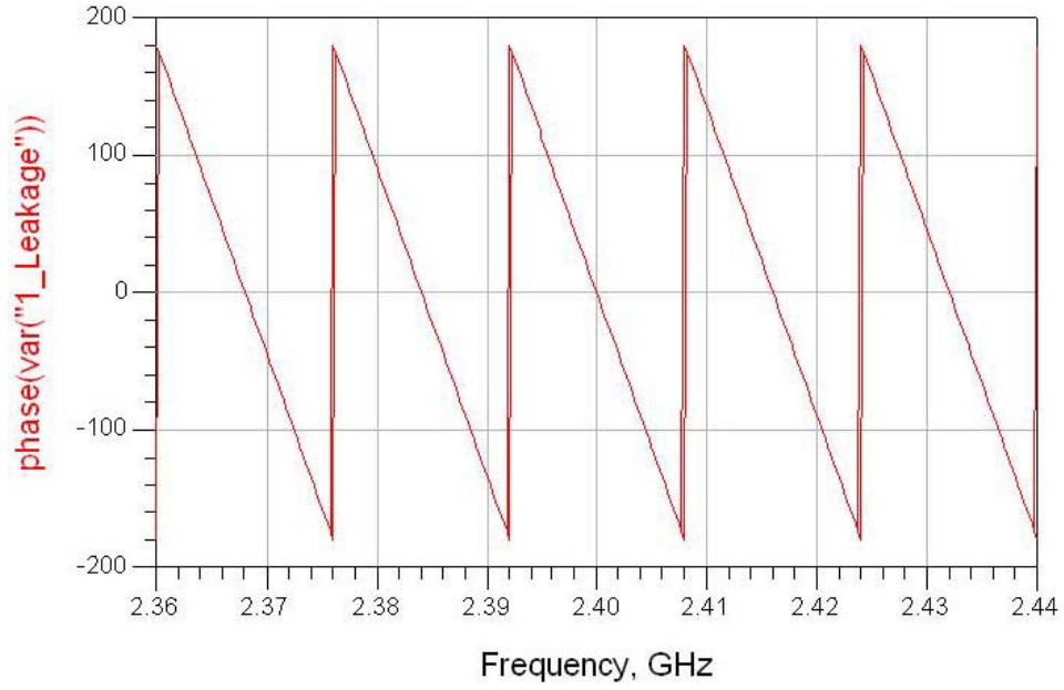
Figure 87. Phase Plot of Leakage in WLCC.
