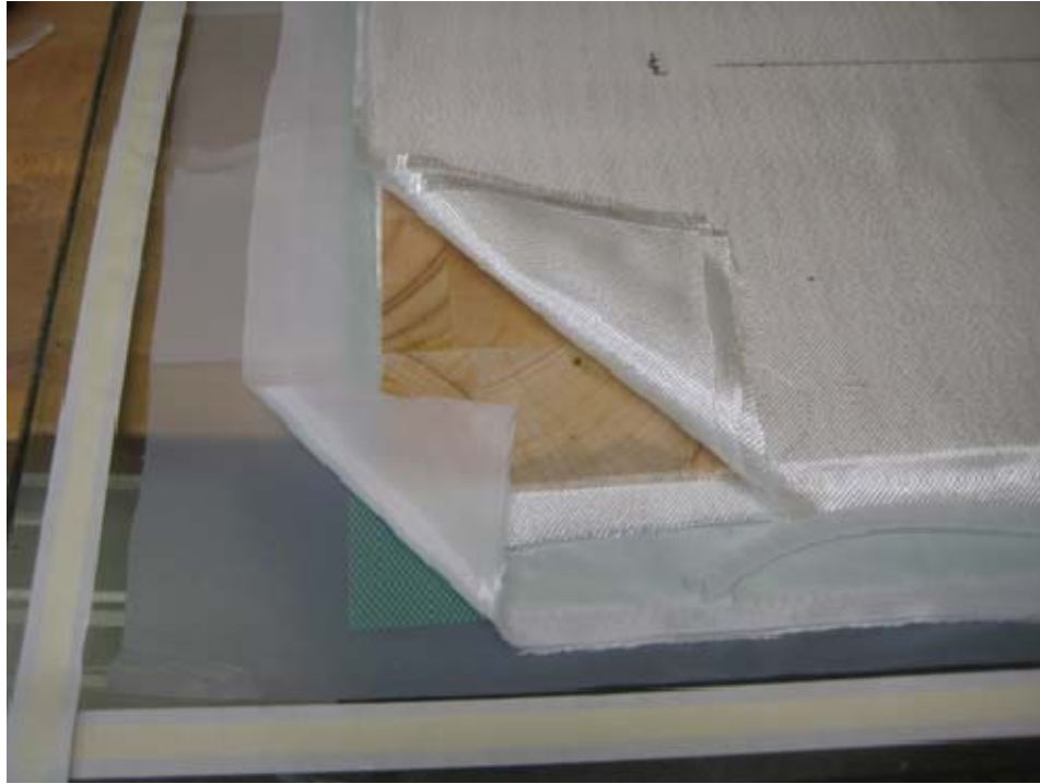
Figure 2. Dry layup, bottom to top: Teflon, distribution medium, peel ply, E-glass, Balsa Core, E-glass. Not yet added: peel ply, distribution medium, vacuum film.
