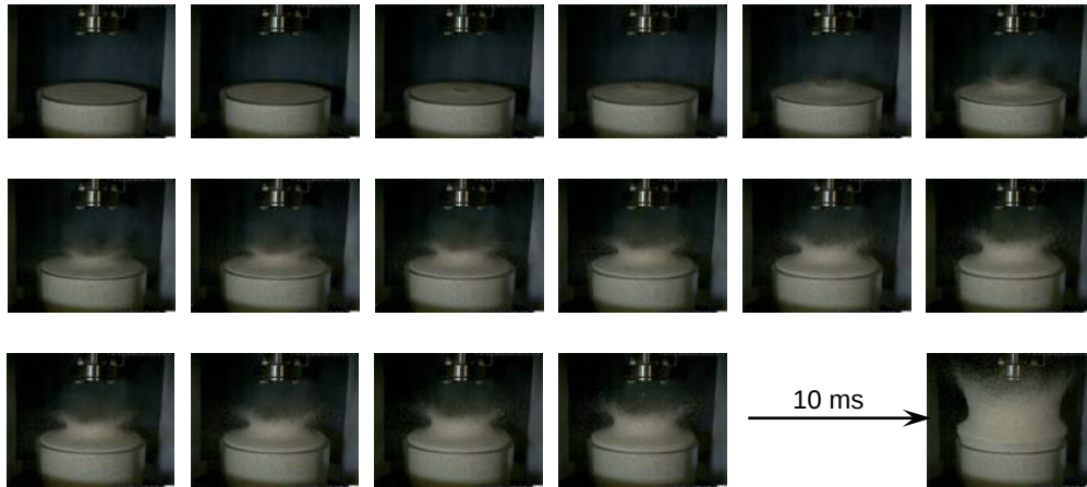
Fig.6 High-speed visualization of behavior of ejecta.
