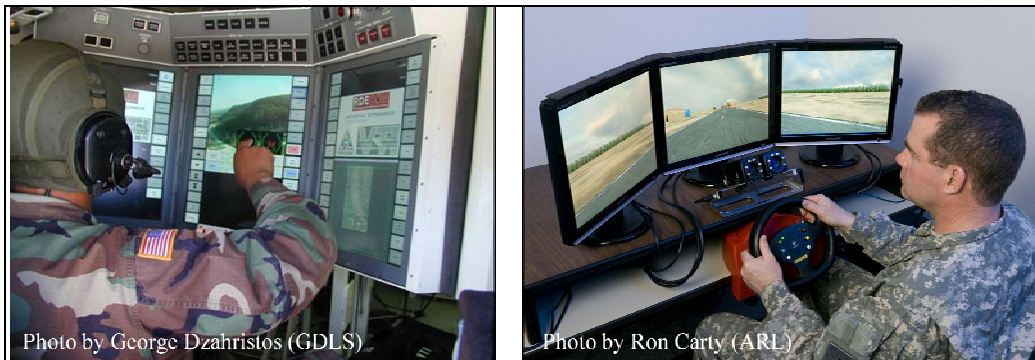
Figure 1. Crew station in CAT-ATD vehicle (left) and CAT-ATD control station simulation (right).
