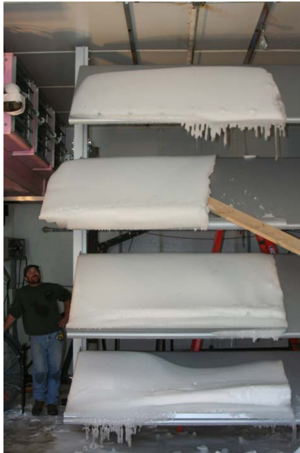
Figure 3.18. Snow mass can be pushed off the end of the fin, providing confidence that the IRDs retain the accumulation in place.
