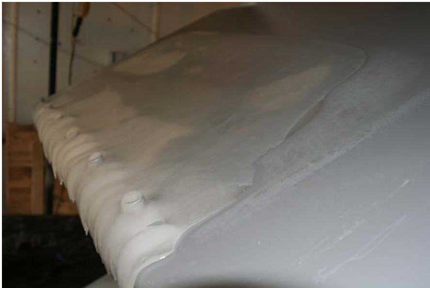
Figure 5.27. Condition of fin A2 after a day of melting with the inverted IRD option 4 protruding through the cover.
