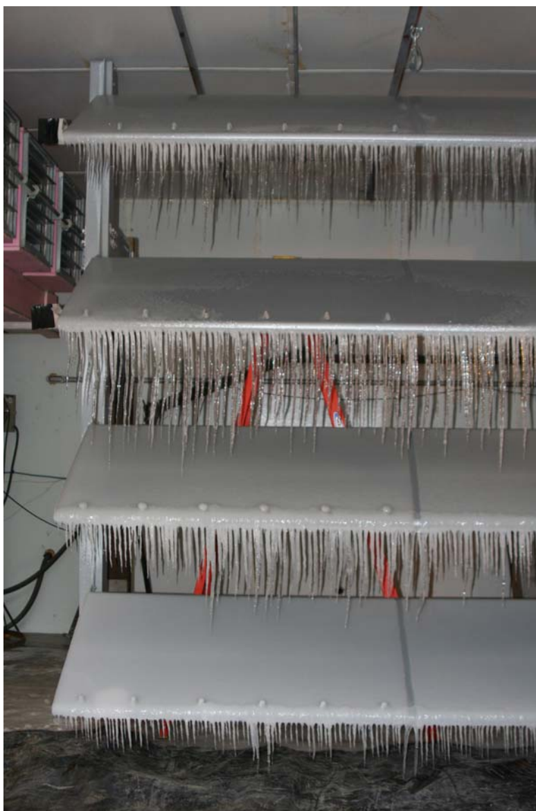
Figure 31. Icing conditions at the conclusion of heating fins A3 and A4 with radiant heaters while shading fins A1 and A2. The room temperature was approximately 23 °F, and the melt water refroze on the lower panels.
