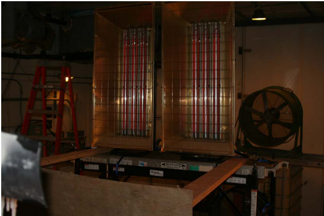
Figure 30. Using radiant heaters to simulate solar heating of the top fins (A3 and A4) while the bottom fins (A1 and A2) are shaded by the plywood.
