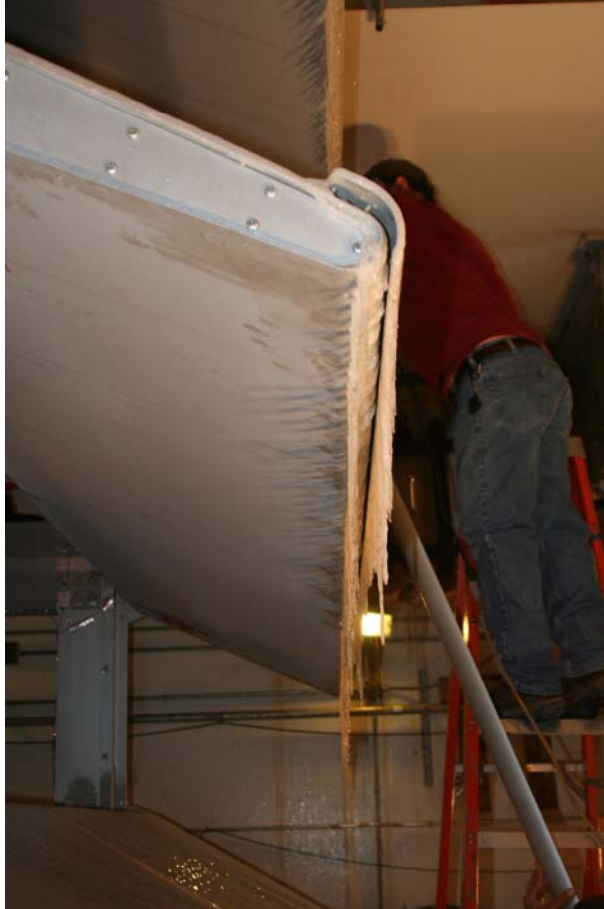
Figure 4.11. Bottom of fin B3 with IRD option 3. The majority of the icicles are attached to the front skin as the water is flowing over the top barrier as shown in Figure 4.10.
