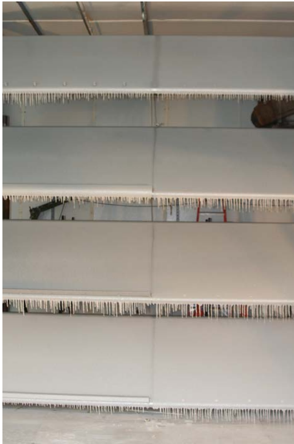
Figure 1.1. Initial conditions of fins with the vertical centerline deiced. The ice retention devices are installed on the A (left) side of the fins. The B (right) side is used as the control. IRD options 1, 2, 3, and 4 are installed on the A side of the fins, starting with option 1 on the bottom fin (A1) and progressing to option 4 installed on the top fin (A4).
