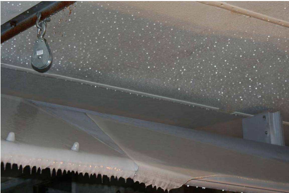
Figure 27. IRD option 4. The buttons 12 inches on center are encapsulated in ice and retain the sheet of ice (left), while the ice slides off without the IRD (right).
