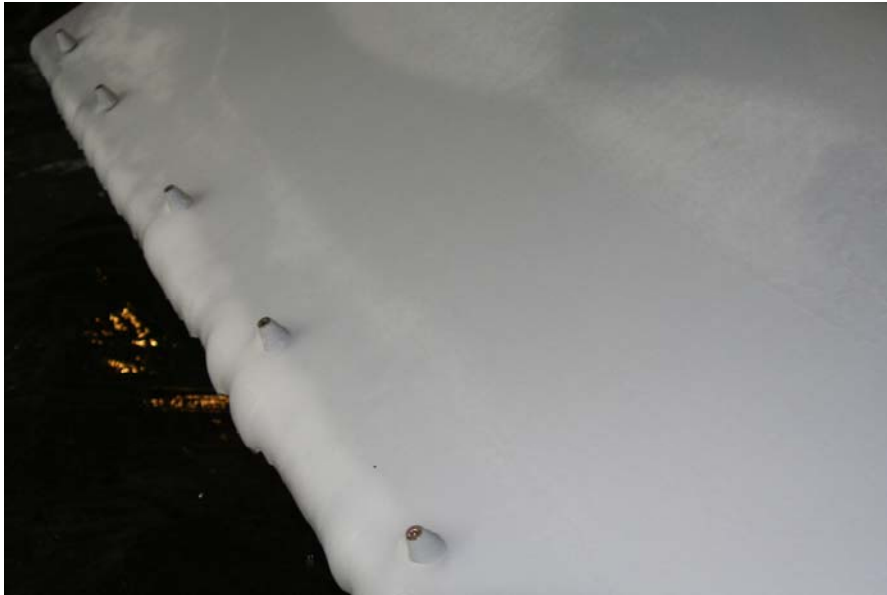
Figure 5.26. Fin A1 after a day of melting with just the IRD option 4 protruding through the ice accumulation.
