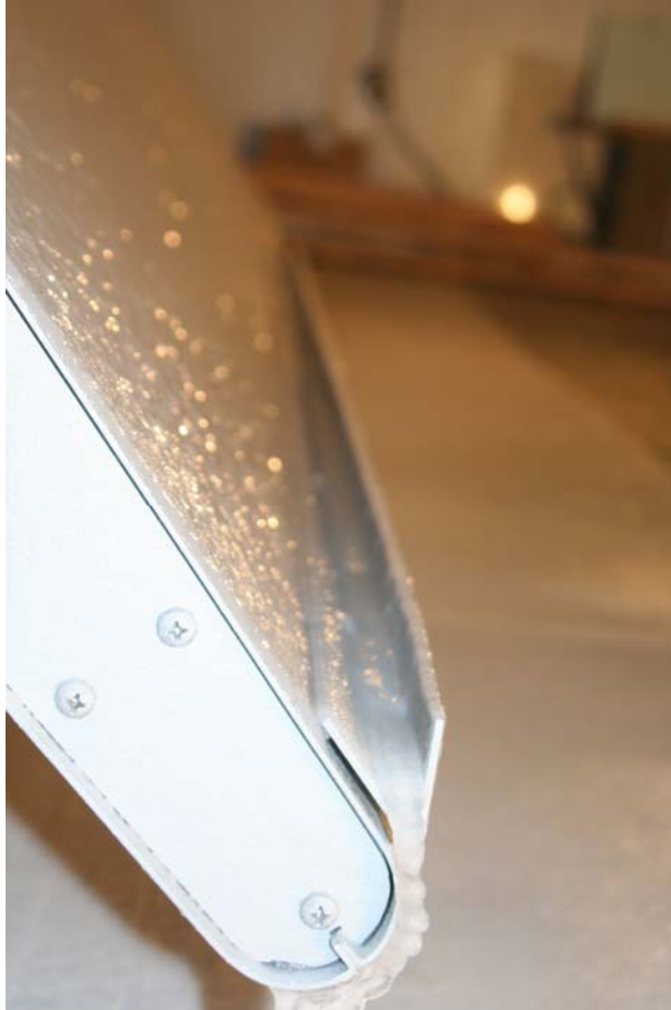
Figure 1.2. Fin A1 with IRD option 1 installed. Note the drainage paths are blocked with ice and the continuous IRD serves as a gutter.
