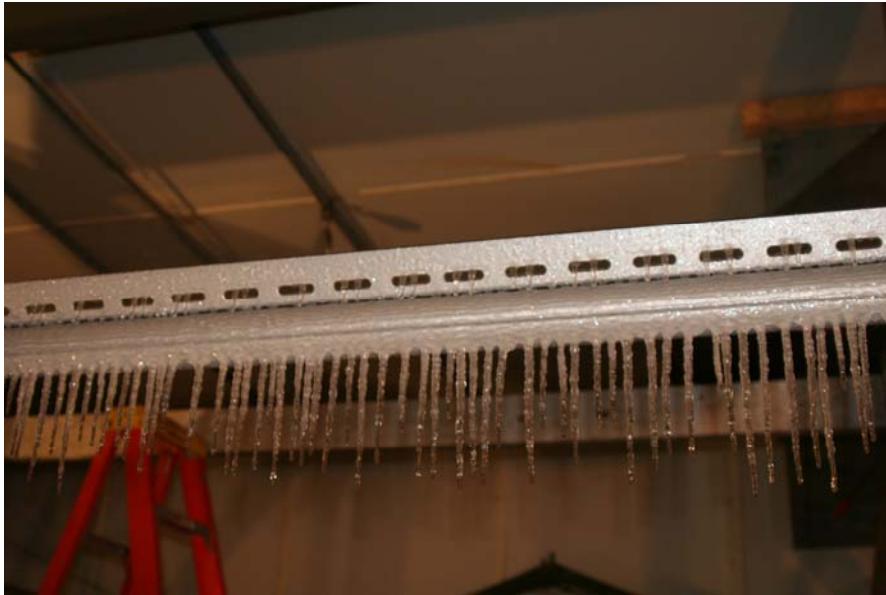
Figure 4.3. Condition of IRD option 3b (1/2- x 2-inch slots 3 inches on centers) on fin B3 after 40 minutes of icing.
