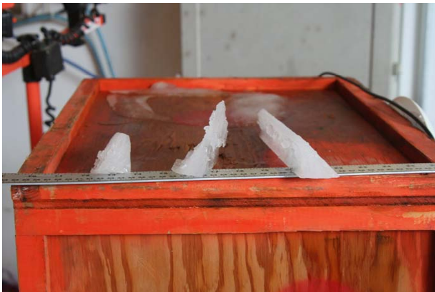
Figure 4.21. Ice accumulation from behind IRD options 1 and 2. Given the volume of ice, considerable melting would have to take place before the drainage paths under the IRDs would be open.
