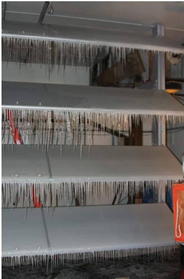
Figure 5.20. Fins on the B side; the radiant heaters on fins A3 and A4 did cause melting on fins B3 and B4.
